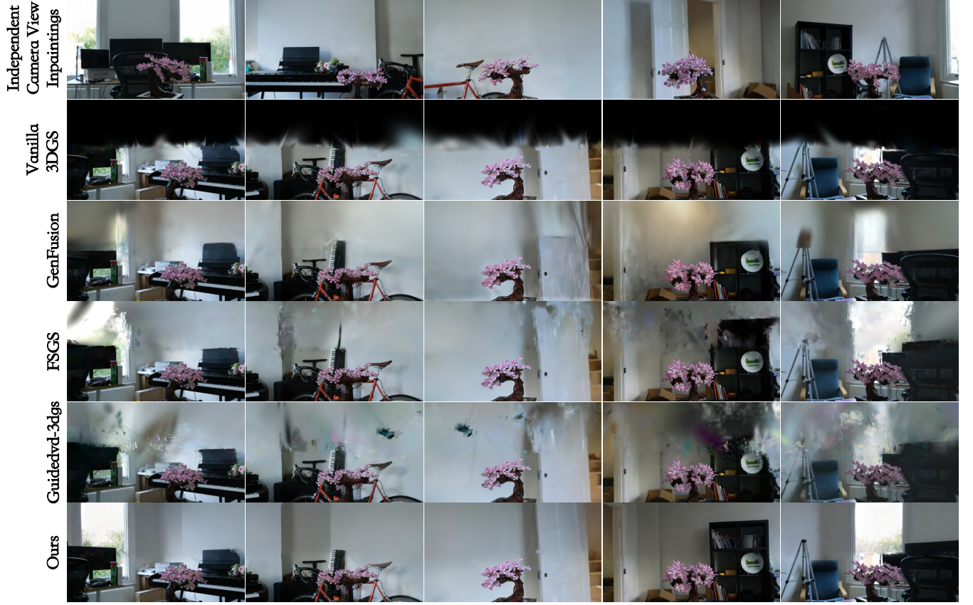
Figure 7: Qualitative comparisons of extrapolation on Mip-NeRF 360. The first row shows the inpainted images on independent camera views V_I . The following rows show the images rendered on the camera views between each pair of V_I^i, V_I^{i+1} . Our framework achieves high rendering quality on extrapolated areas while also leaves well-reconstructed original areas untouched.
